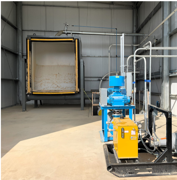
Wood Receiving Hopper with a PD Blower & Hydraulic System. Designed and Commissioned by CMT
