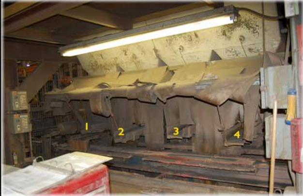
4 Volumetric Vibratory Pan Feeders Problems: Material Flow, Dust Control, Feed Rate Accuracy, Sand Loss
