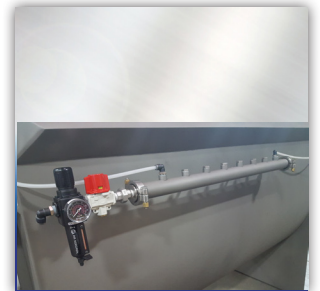
CO2 tangentially mounted injection nozzles and manifold
