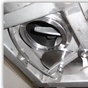
Manually actuated paddle gate
