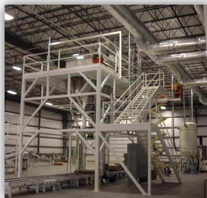
OptimaBlend® production blender for preparing flour mixtures.
