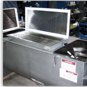
Tailored blender covers for hand dumping and easy cleanability
