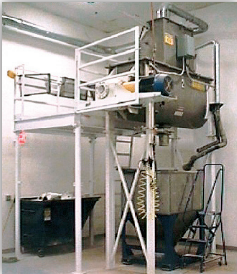
Typical semi-automatic system set up with bag dump and blender into intermediate bulk container (IBC). Later, the IBC to be moved above packaging operation
