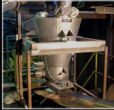
(1) GeoMate™ Feeder to feed 4 - 55 PPM Weight Based, Self Monitoring No moving Parts
