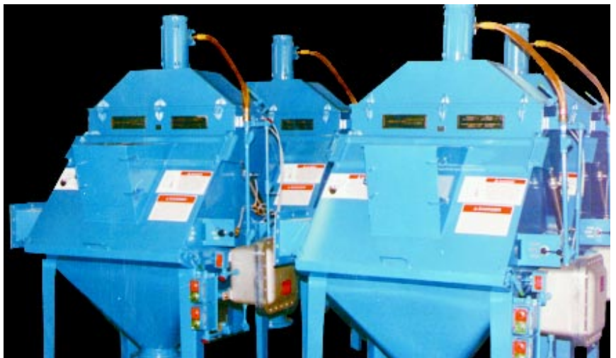
Carbon steel work stations for supersack dumping via spout on front of door.
