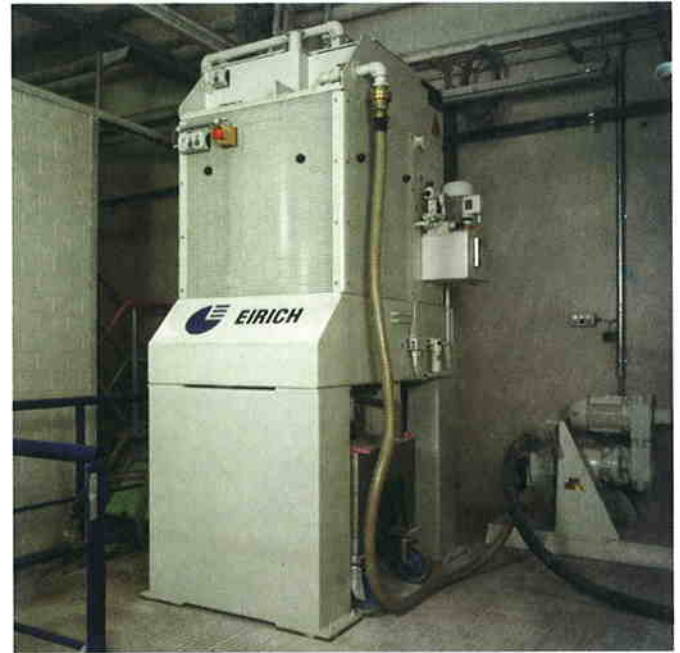
MaxxMill® MM3 for the wet grinding of slip
